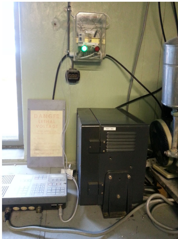
LLE-4 Radio Northern Star, from an ex-Marine Skanti TRP-8250 HF 250 Watts remotely controlled transmitter at LKB/LLE Bergen Kringkaster broadcasting on 1611 khz with @70 watts AM and 250 watts USB.
