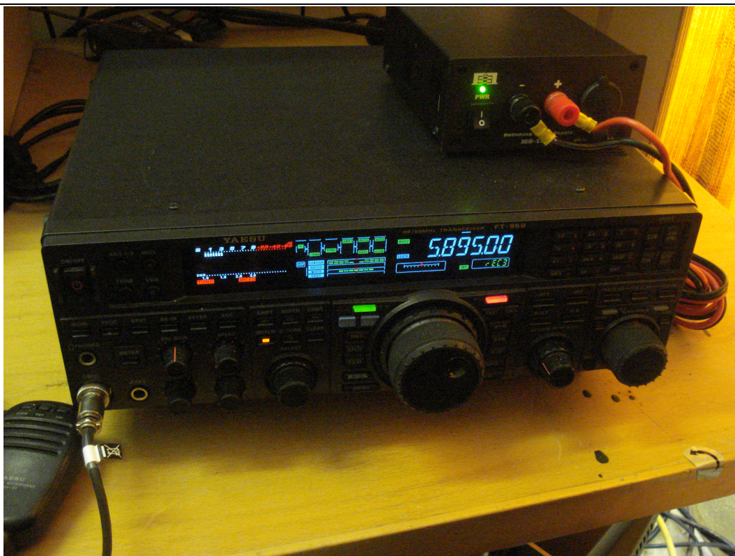
LLE-3, Radio Northern Star, from a converted Yaesu FT-950 25 watt AM, 100 watt USB transmitter, broadcasting from LKB/LLE Bergen Kringkaster in the 49 metres SW band, 5895 kHz.
